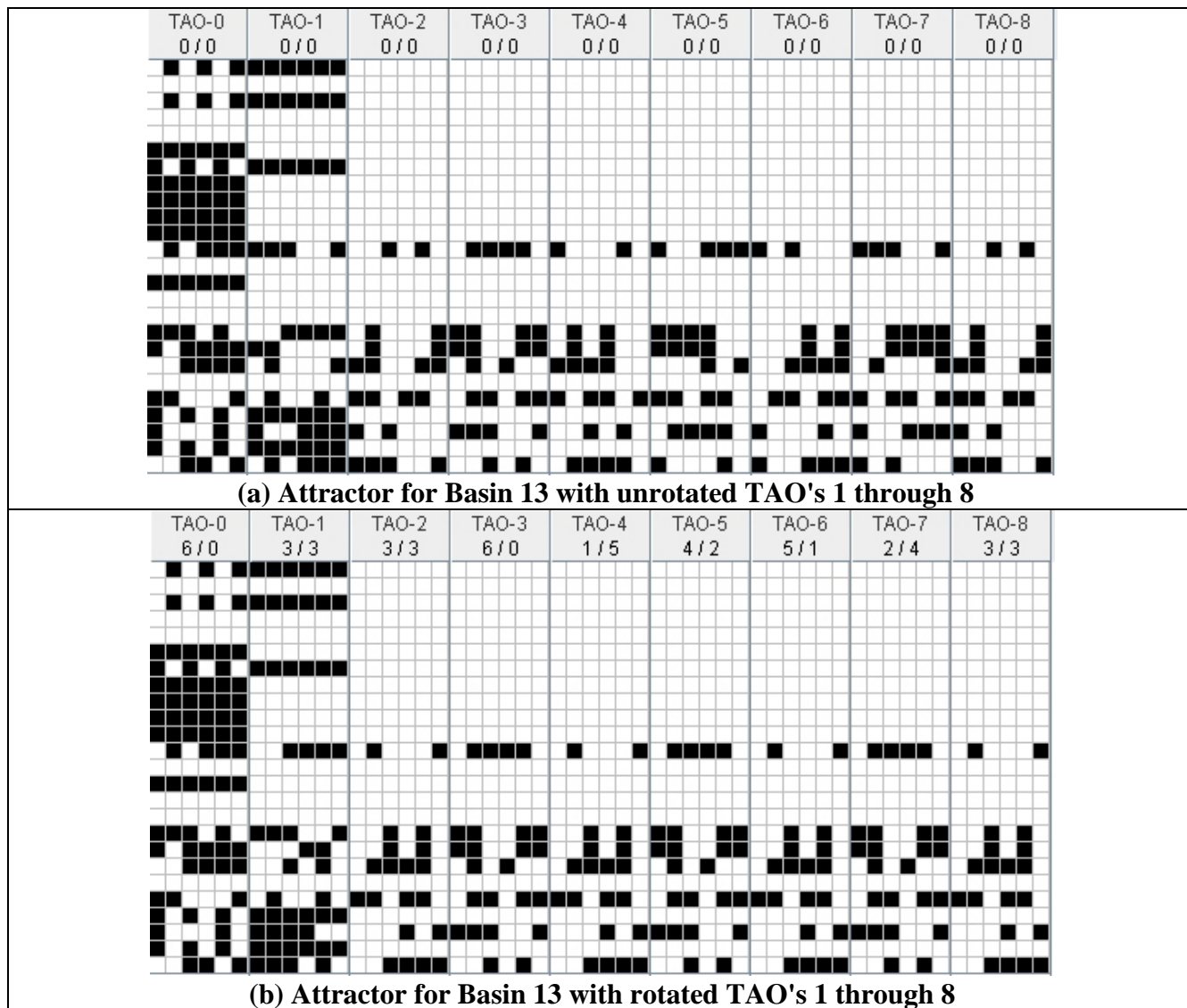
Figure 1.6. A single attractor cycle for Basin 13 for a small Boolean system with N = 25 nodes. The original attractor cycle is labeled TAO-0 and the figure shows that individual nodes whose sub-cycle is a power of 2 (e.g., top node alternates ON-OFF and thus has a sub-cycle of L=2 ) resolve to a vector of 0's (all white) with recursive applications of TAO while nodes (e.g., bottom node) do not resolve to 0 .
