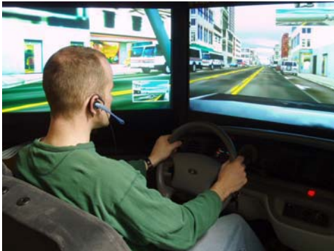
Figure 1. A participant talking on a cell phone while driving in the simulator.
